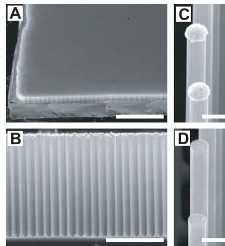
**Fig. 1.** (A) Scanning electron microscope image showing the p-Si wire arrays on a  $\sim 2\text{-cm}^2$  wafer (scale bar,  $600 \mu\text{m}$ ). (B) Side view of a cleaved sample (scale bar,  $50 \mu\text{m}$ ). (C) Close-up showing the faceted wire and the copper catalyst tip before etching (scale bar,  $2 \mu\text{m}$ ). (D) Close-up showing the wire tops after etching with  $\text{FeCl}_3$ ,  $\text{KOH}$ , and  $\text{HF}$  (scale bar,  $2 \mu\text{m}$ ).
