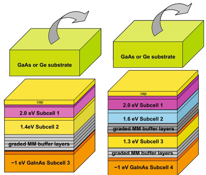
Fig. 7. Schematics of an IMM 3-junction and an IMM 4-junction concentrator cells.
