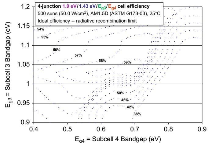
**Fig. 4.** Dependence of ideal efficiency on Subcell 3 and Subcell 4 bandgaps,  $E_{g3}$ , and  $E_{g4}$ , for a 4-junction terrestrial concentrator cells limited by radiative recombination at ~500 suns.
