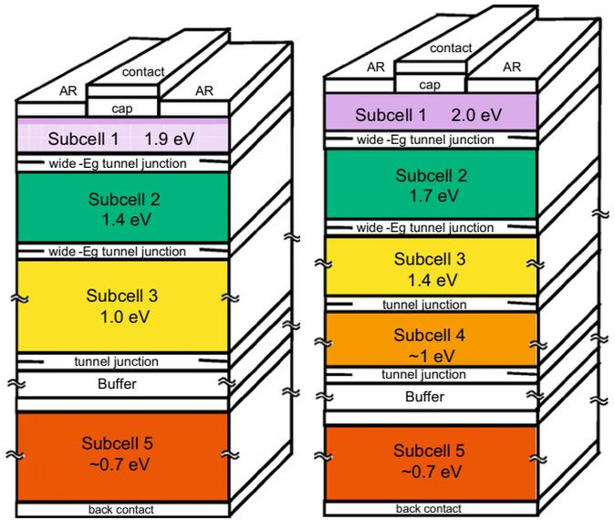
**Fig. 3.** Schematics of a 4- and a 5-junction concentrator cells.
