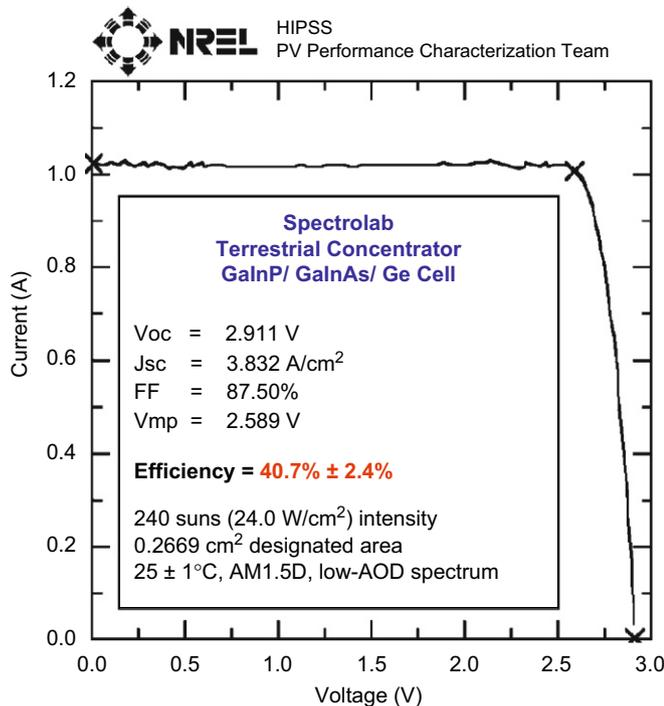
**Fig. 2.** Illuminated *I-V* curve of the 40.7% 3-junction cell certified at NREL.
