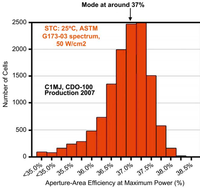
**Fig. 1.** Efficiency distribution of approximately 13,000 1 cm<sup>2</sup> Boeing-Spectrolab terrestrial concentrator cells tested at ~500 suns. The cells have a mode efficiency of 37%.
