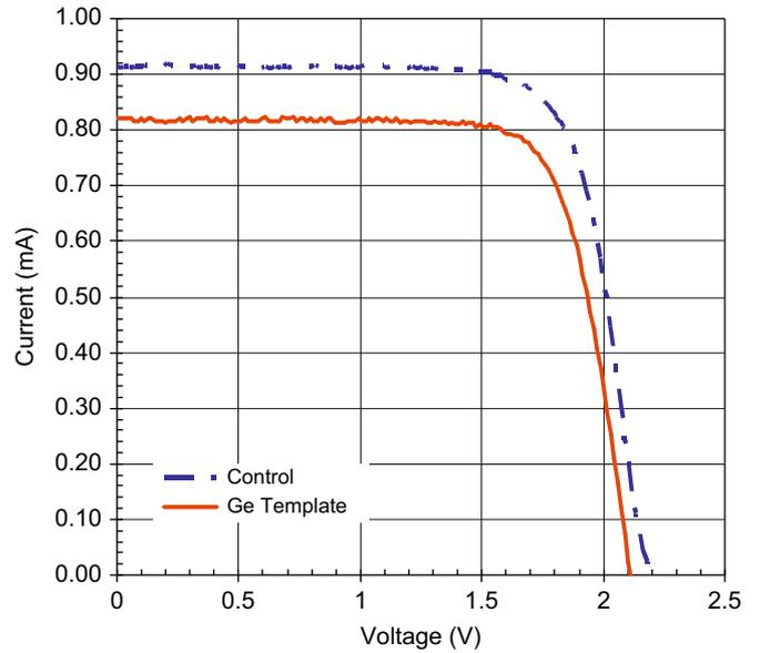
Fig. 10. Measured I–V characteristic of a control 2-junction cell and a wafer-bonded, layer-transferred 2-junction cell under the AM1.5G Spectrum (cell size = 7 mm<sup>2</sup>).
