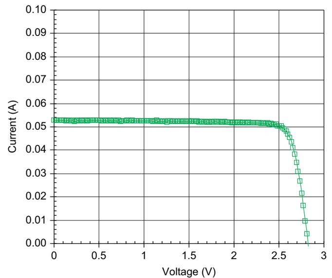
Fig. 8. Illuminated  $I$ - $V$  characteristic of an IMM 3-junction cell tested at 7 suns under the AM1.5D spectrum.
