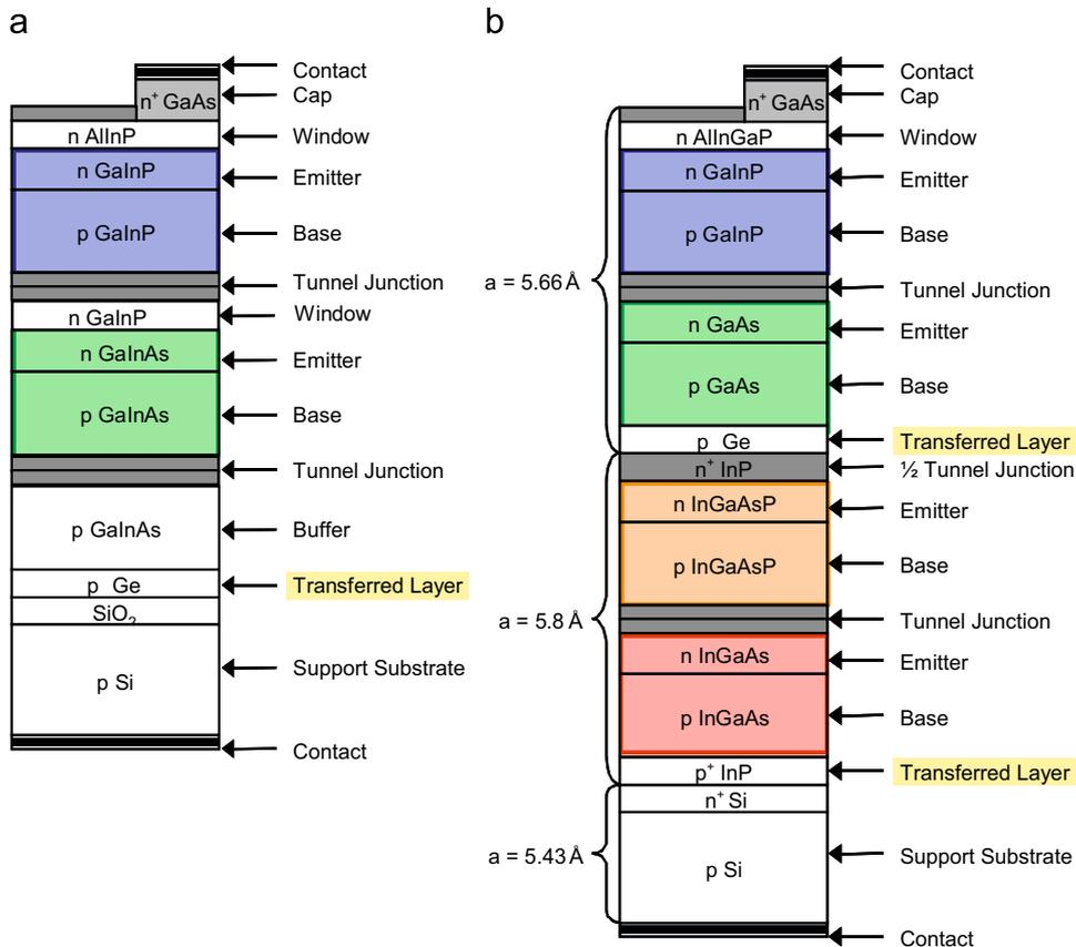
Fig. 9. (a and b) Schematics of the demonstrated 2-junction cells and the final wafer-bonded, layer-transferred 4-junction cell.
