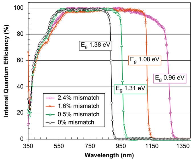
Fig. 5. IQE curves of metamorphic  $Ga_{1-x}In_xAs$  single-junction cells with bandgaps ranging from 1.38 to 0.95 eV.
