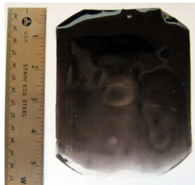
Fig. 5. Photograph of a polymer-embedded microwire array.
