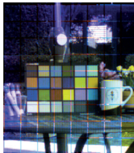
Figure 1 | An image captured using a commercial CMOS camera but with a plasmonic colour filter array instead of the standard dye-based one, after full computational reconstruction and signal processing. Reproduced with permission from ref. 12, © 2013 American Chemical Society.
