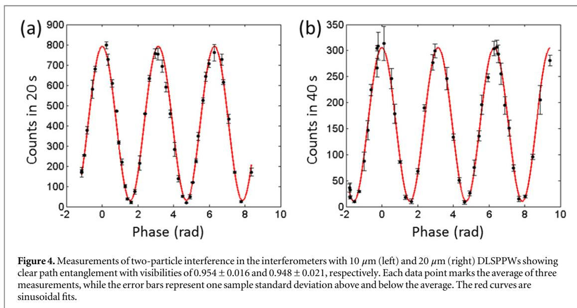
result is nearly identical to that in panel (a), indicating that increasing the length of the DLSPWs (and therefore the losses suffered) did not affect the degree of path entanglement.
